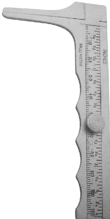
M-1209-00 Wills Bit Gauge Scale 0.100mm Both side Graduation
